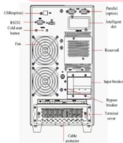
10-40kVA UPS with battery space
